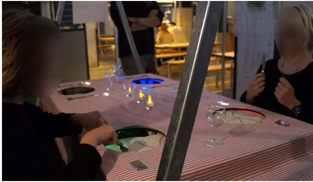
Figure 2: The Hunger Games installation. The aperture on the left is closing and the aperture on the right is already closed. The conductive sensor that can detect the presence of cutlery can be seen next to the apertures (grey areas).
